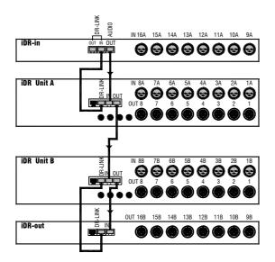
**Expanded multiple iDR system** This diagram shows an iDR system with two **iDR-8** units and both expanders fitted. A system could also be created with **iDR-4** units or a mix of **iDR4** and **iDR-8** units. DR-Link is only required to connect to the expanders, not between the main units. Make sure you connect DR-Link to the **iDR** associated with each expander. Make sure you plug into the correct DR-Link socket. In this case do not daisy chain DR-Link from one expander to the other.
